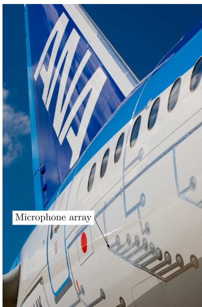
Fig. 1 Boeing 777 fuselage instrumented with an array of microphones. (Courtesy Boeing.)
